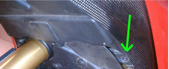
Depress tab and separate harness from sensor.
