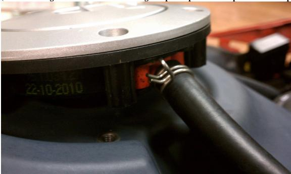
With the cap loose you can leave the left hose and optional wire for keyless caps attached and hang the cap over the handlebars out of the way.
