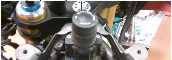
Remove the 2 screws holding the HFCU.
