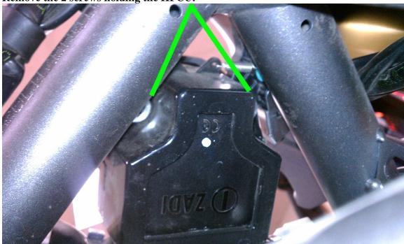
Remove the wiring connectors to the HCFU:
