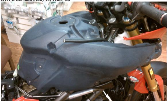
To remove the tank, lift the rear and then lift the front slightly and pull the tank to the rear. It will have to come up slightly to clear the frame.
