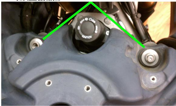
Remove the 2 lower tank mount bolts: Two 4mm hex screws
