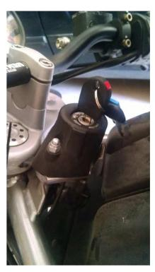
Remove 2 10mm nuts securing the black plastic aerial cover over the ignition lock assembly
