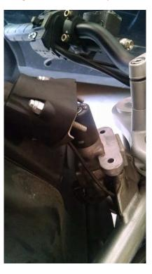
Sometimes the nut and stud will spin loose together (pictured above right). If this happens on both studs it may make your job a little easier. Just remove the aerial and studs together and then hold the studs with a pair of vise-grip pliers (do not damage threading) to remove the nuts with a socket.
