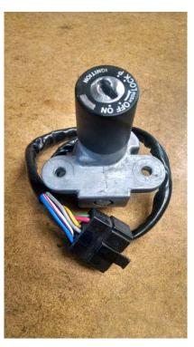
When reinstalling the lock, use a drop of thread locker on each of the 4 sets of threads to prevent the studs or nuts from coming loose with vibration.
