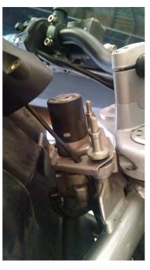
Using locking pliers, grip the stud base firmly and turn it counterclockwise to remove it. Again, be careful not to damage the aerial wire with the pliers. Remove both studs.
