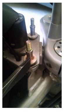
If you have trouble with the locking pliers, another method to break the studs loose is pictured left using a chisel and hammer to loosen the stud. Angle the chisel slightly in the direction you want to turn the stud and strike it firmly to get a good "bite" on the metal. Strike the wider base of the stud. After getting the stud to turn slightly with this method, you can continue with the locking pliers.
