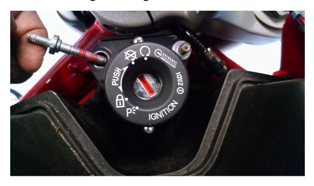
2 studs and lock removed
