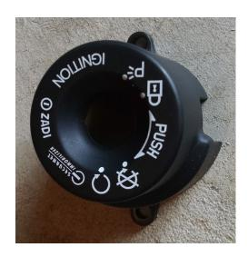
Next you need to remove aerial ring attached to the wire on the left. There is a small horseshoe shaped clip holding the wire in place. Remove it before pulling the aerial ring up and off of the lock. (photo is of a lock removed from bike)
