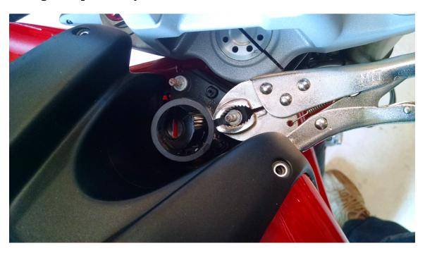
Optionally, to give yourself more room to work, you can remove the black plastic cover from the gas tank retained by 11x 3mm hex screws.
