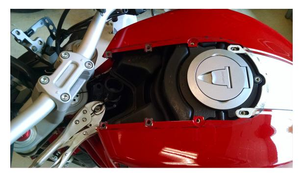
Once loosened, the stud can be turned with standard pliers or without locking the pliers (as pictured below)
