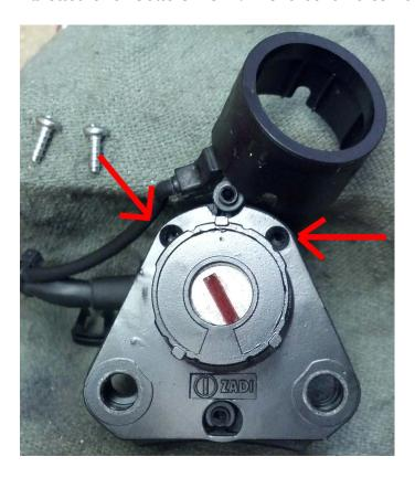
Next remove the black metal cover holding the lock cylinder in the housing.
