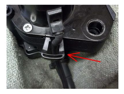
Lift and remove the aerial antenna ring and let it hang off to the side. Be careful not to stress or kink the wires. This is the antenna that picks up the signal from your programmed keys.
