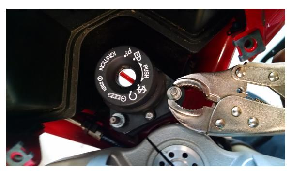
Here is one stud removed. You can see the red thread locker adhesive used to retain the stud. When reinstalling, it is recommended to use thread locker to prevent unwanted loosening while riding.
