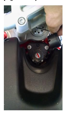
Using a good quality pair of locking pliers, adjust them to lock on the stud base (careful not to damage the threaded portion) and rotate counter-clockwise. Do not damage the paint on your handlebars.
