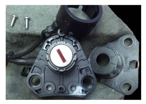
With the cover removed the lock cylinder is free to be pulled out.
