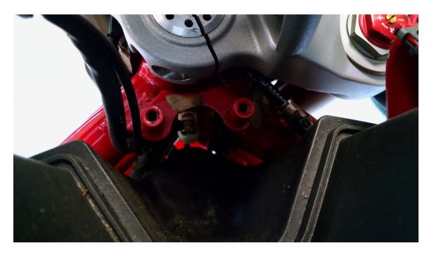
This is the white plastic harness connector for the ignition switch. Unlock and disconnect it and then cut any nylon ties holding the wire to the frame to remove the lock and switch.
